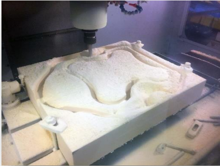
Figure 7: Blocks of Polyurethane Foam Boards glued together
