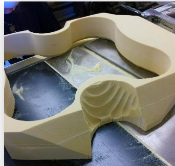
Figure 8: Bottom Float Prior to Sanding
