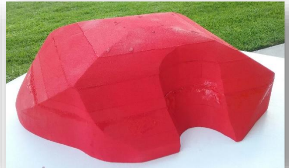
Figure 9: Finished Float Prior to Resin Coating
