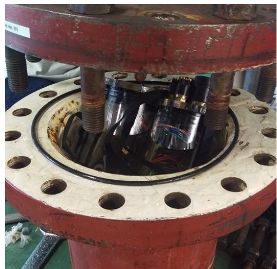
Pressure test chamber used for testing dry housing
