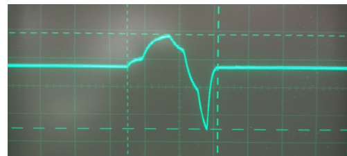
Oscilloscope capture, with 85\text{mF} of capacitance, showing a small 50\text{ms} , 0.5\text{V} spike, with the regulators continuing to function
