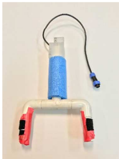
Figure 25 Valve Turner (By Gavin Chan)
