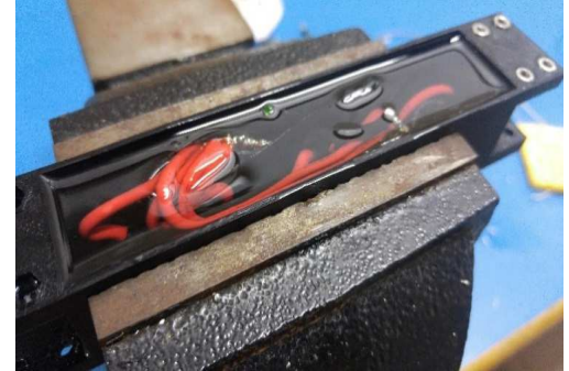
Figure 32 Power bar filled with epoxy (By: Joshua Ho)
