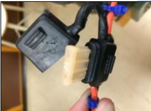
Figure 4: A 25A fuse inside fuse holder on positive lead. (Credit: Mitchell Tuck)
