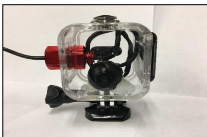
Figure 24: CarRover backup camera with a GoPro waterproof housing. (Credit: Raquel Morgan)
