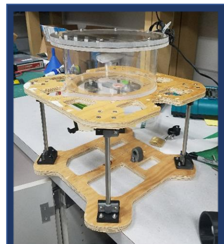
Figure 2.1 Plywood ROV prototype
