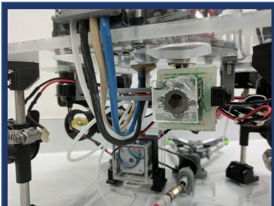
Figure 2.6 Waterproofed, and mounted camera
