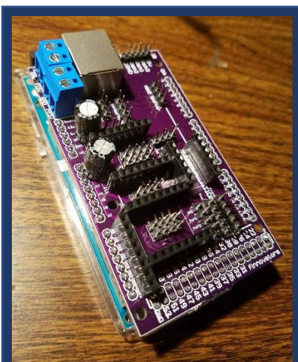
Figure 2.16 Custom shield attached to Arduino Due
