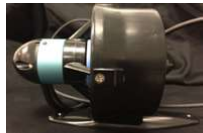
Blue Robotics T200 Vertical Thrusters
