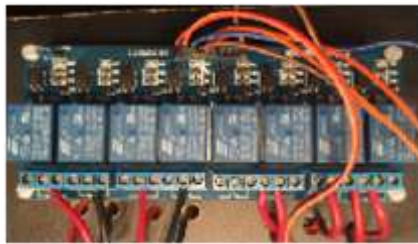
Relay board in control box
