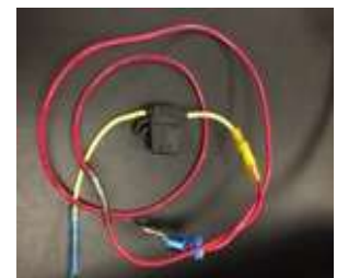
25 Amp fuse connected in main power line.
