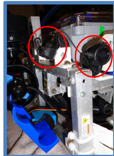
Figure 11: Cameras Mounted on Frame
