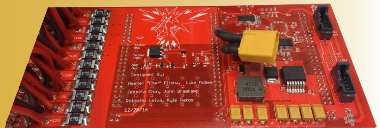
Fig. 29 - Power Distribution Board
