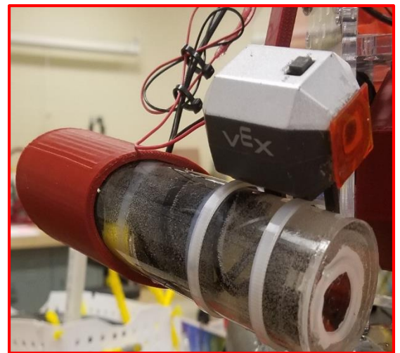
Raman Laser secured to exterior of secondary camera.
