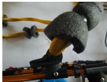
Strain relief on tether on ROV side.
