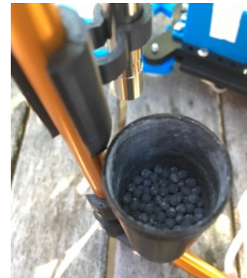
3D Printed capsule for shotgun pellets. (Photo Credit Walton)
