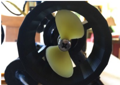
Lateral motor with a 3D printed motor shroud. (Photo Credit Walton)
