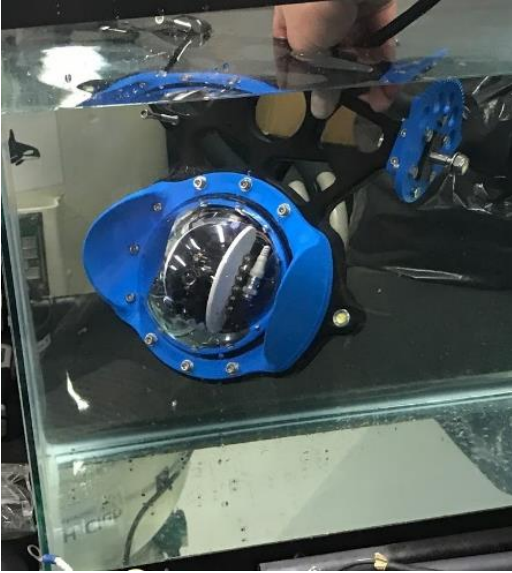
Figure 16: Camera Water Test Photo Credits: Gunnar Hoglund
