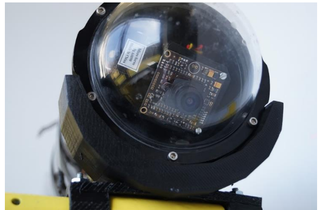
View of the dome end cap on our electronics housing. *Photo by Kelly Cool
