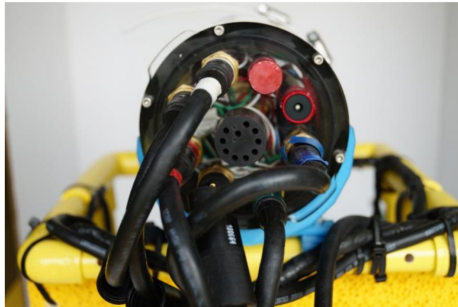
Rear view of the ROV, showing the SEACON connectors.
