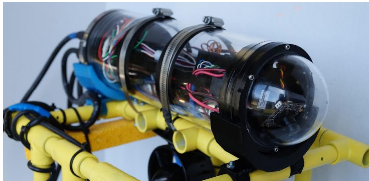
Front view of the ROV, showcasing the dome endcap. *Photo by Kelly Cool
