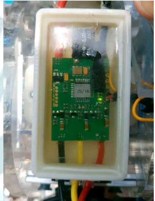
Figure 9. Electronic Speed Controller sealed with the 3D printed case filled with epoxy resin.
