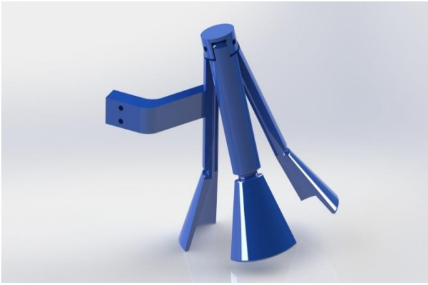
Picture 5. 3D model of rebar holder
