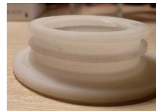
Figure 6 Resin 3D Printed End Cap. Captured by Marwan.
