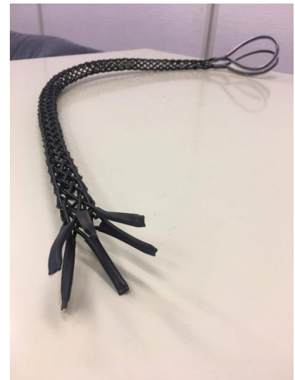
Figur 13: Strain-relief to protect the tether.
