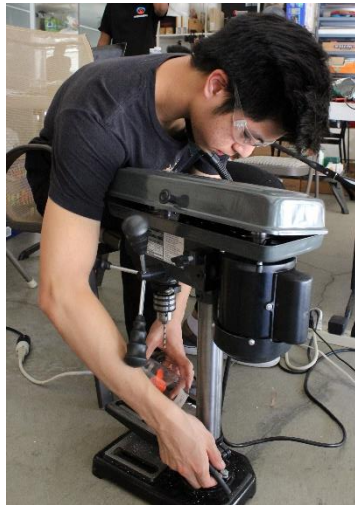
Figure 2: Member wears safety goggles to protect eyes from plastic that may fly off while drilling.
