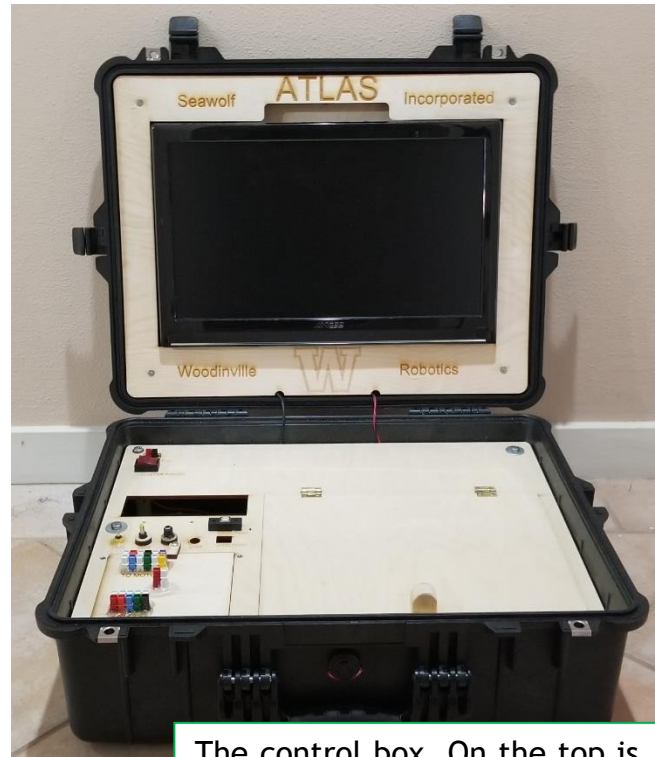
The control box. On the top is the monitor. On the left is the I/O, and on the right is storage.
