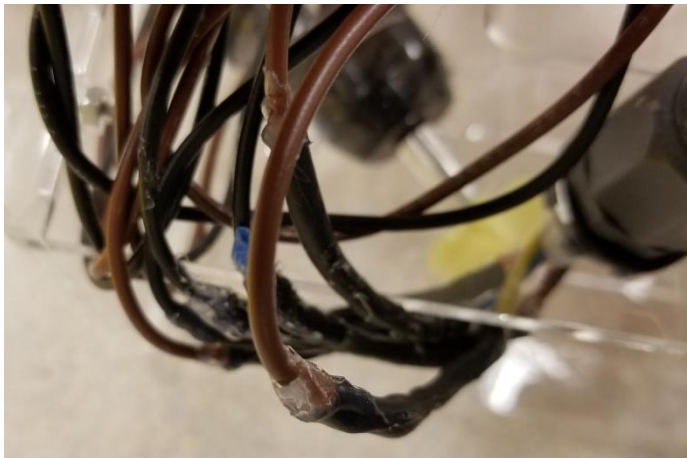
The motor wires on the Atlas. The clear hot glue and black heat-shrink tubing are visible around the joints.
