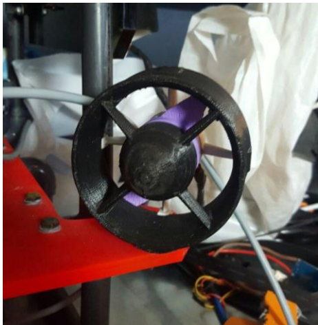
Figure 19 - 3D printed Nozzle
