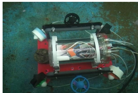
Figure 30 - Initial version of ROV in stability tank test
