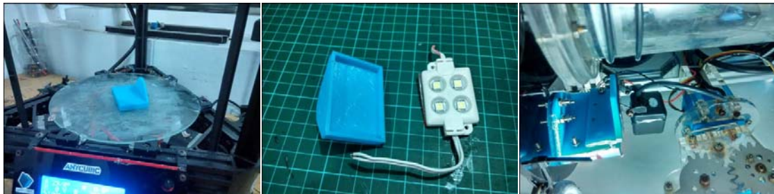
Figure 16: Make holder from 3D print, and place to side robot (Credit: Dendy.)
