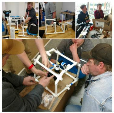
middle, which are holding the 2 of 4 motors, to make it more compact. This will allow the Engineering Personnel, Quintin and Gavin, constructing the frame. ROV to traverse the confined and precarious locations typically connected with underwater crashes and maneuvering around the Debris. Towards the beginning, the frame of the ROV was uneven, so we had to take it completely apart and rebuild; However, this provided us with another chance to explore possibly better ideas.
