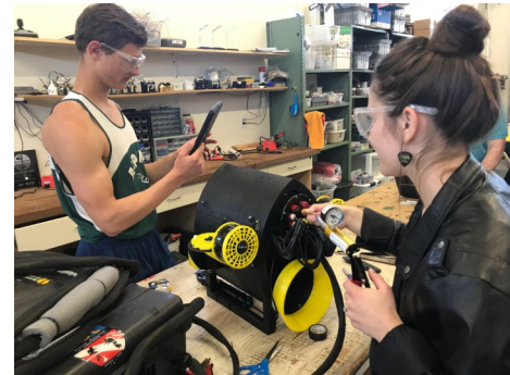
(Above) Eva Lusardi checks the enclosure pressure while Wenton Harris records the measurements.
