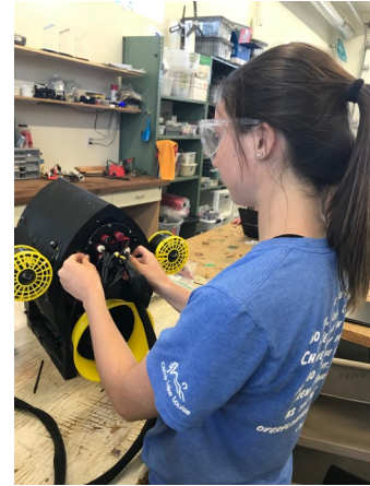
(Above) Abby O'Brien check the enclosure for any air leaks.
