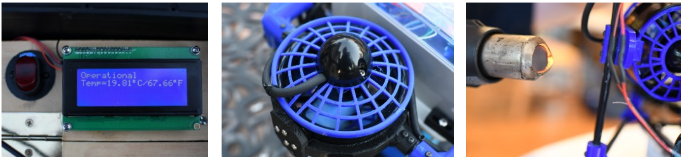
(Left to Right) Leak detector in the control box; 3D printed motor shroud; waterproof heat shrink used on all splices
