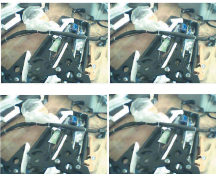
Figure 13: (From top to bottom, left to right) Raw image, Gaussian Blurring, Median Filtering, and Bilateral Filtering applied sequentially on the frame. Each filter applied gradually blurs the image, carefully retaining important feature information such as vertical and horizontal edges, but removing unimportant intricacies that can lower the performance of contour detection.
