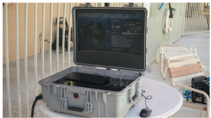
Figure 6B: Top Side Control Box
