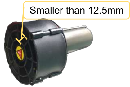
Figure 40: All propellers are shrouded with 3D-printed shrouds (Image by Terry AU)
