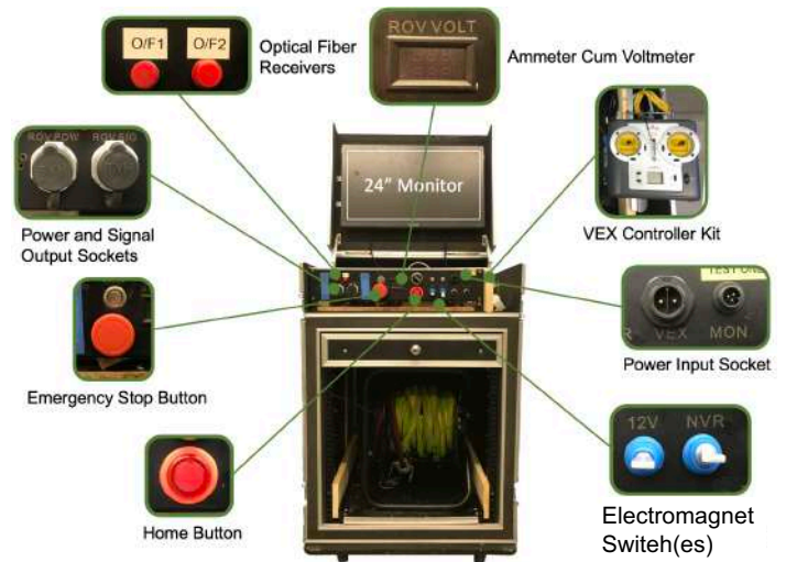
Figure 14: Features of the EDCP (Image by Terry AU)
