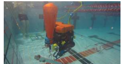
Figure 30: Lift Bag inflating for removing cannon to the surface (Image by Beth AU)
