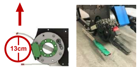
Figure 27: CAD model with Autodesk Fusion 360 and demonstration of Theta 's secondary manipulators (Image by Beth AU)
