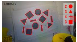
Figure 33: A screen capture of ShapeRecognition's interface (Image by Jerry LUM)
