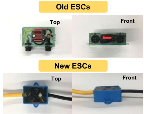
Figure 15: Overview comparison of old and new ESC Boxes (Image by Beth AU)
