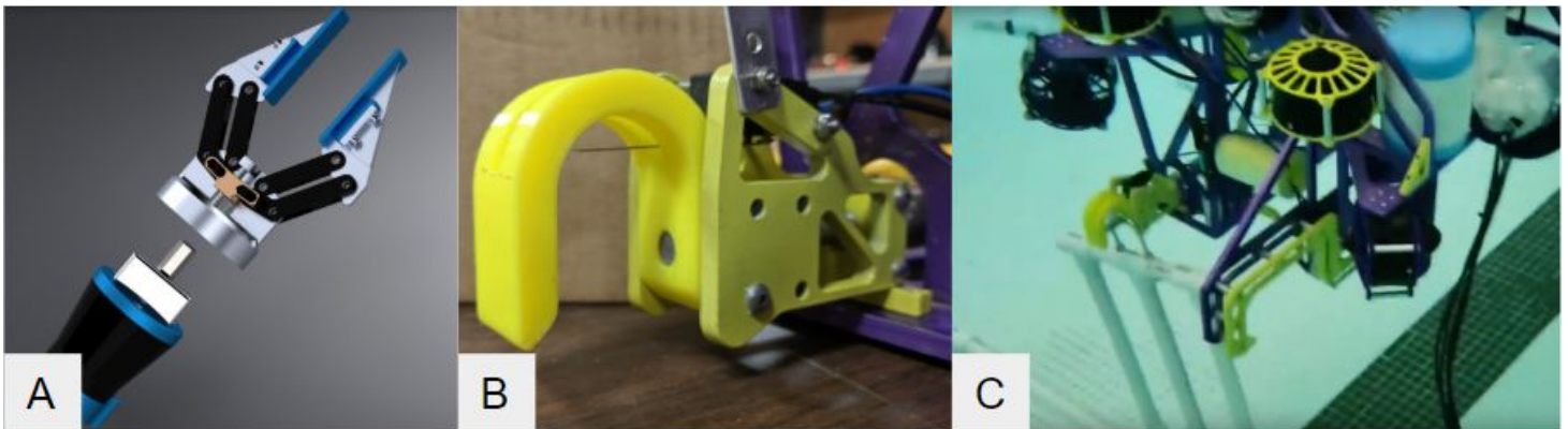
Fig. 15: Manipulator development process.
