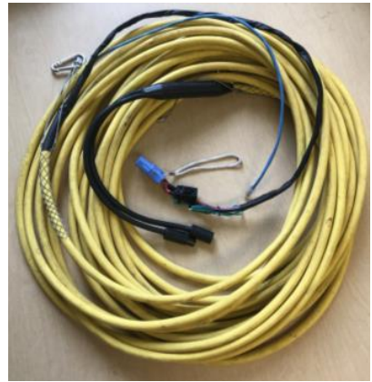
Figure 18: Outland Tether modified for Seawolf VIII
