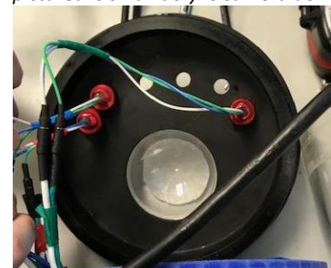
Figure 6: End cap of HDPE. Also pictured is small acrylic camera dome.
