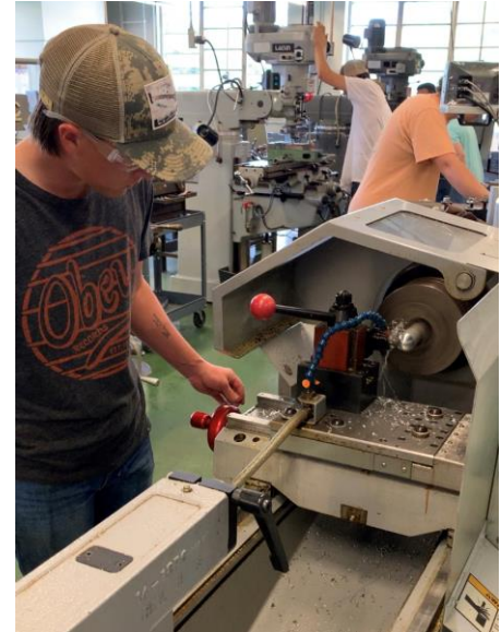
Figure 7: A SURE technician constructing ROV feet on a CNC lathe.
