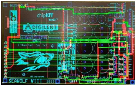
Figure 15: Seawolf VIII Main board from NI Ultiboard Software.
