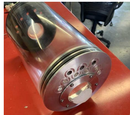
Figure 14: Seawolf VIII acrylic tube and the main rear ROV end cap.
