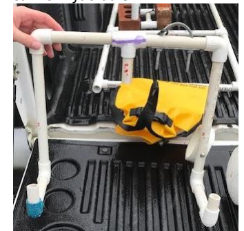
Figure 11: Custom designed cannon lift cradle.
