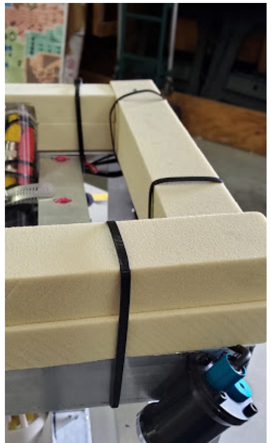
Figure 18: R-33 Subsea Buoyancy Foam mounted on the ROV according to the calculations.
