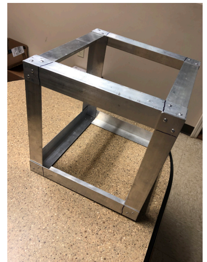
Figure 4: Image shows 38mm by 304.8mm by 4.2 mm aluminium constructed into a cube as the frame of Próklisi. Photo Credit: Ashlee Wall
