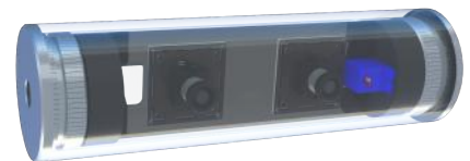
Figure 8: Stereo camera in watertight enclosure with rotation mechanism
