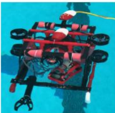
Figure 19: Testing the buoyancy of our ROV
