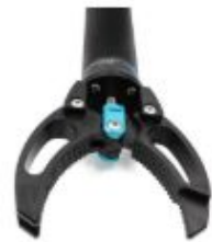
Figure 8: Blue Robotics' Newton Subsea Gripper
