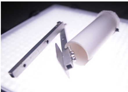
Figure 25. Trout fry dispensing mechanism
