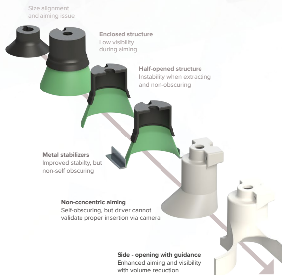
Figure 39. Design evolution of the pH manipulator
