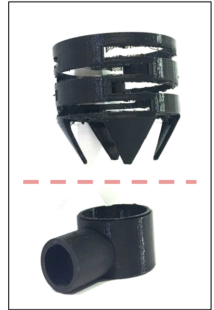
Figure 32. Broken Shroud Photo Credit: Saketh R.
