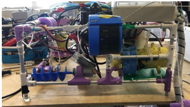
Fig 1.4 Side View of ROV with Micro-ROV
