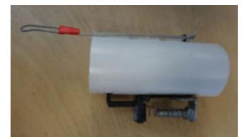
Fig 3.17c Releasing grout device
