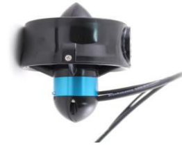
Fig 3.9 Thruster without protection.
