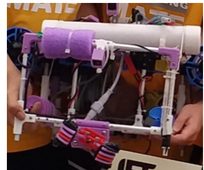
Fig 3.4b Buoyancy supported by plastic boxes, PVC pipes and foam
