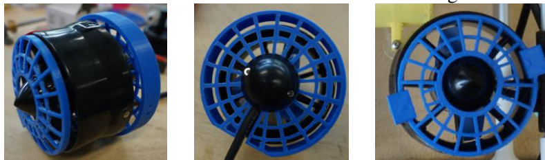
Fig 3.10 3D-printed protective cover guards for both sides (Photo credit:Sam Wong)
