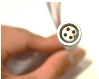
Fig 3.16a Waterproofed plug (cross section)
