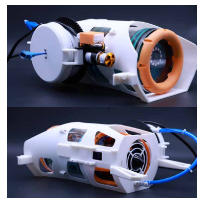
Figure 19. Micro ROV in the silo with the tether wheel attached on top.
