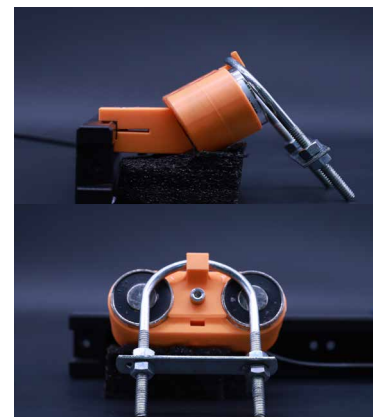
Figure 13. Angled Bi-electromagnet with U-bolt hooked on it.
