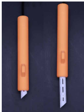
Figure 21. The pH probe retracted (left) and extended (right)
