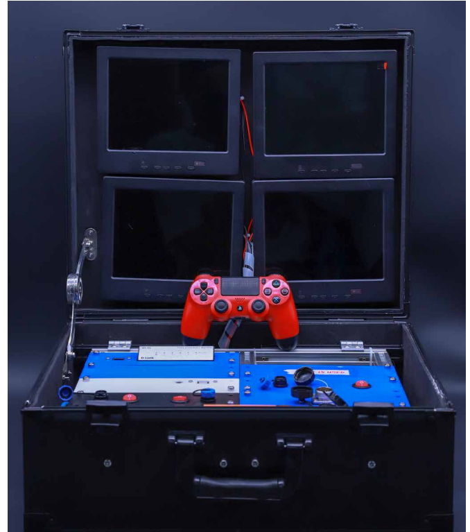
Figure 9. Control box with four monitors on the top, and the module racks on the bottom.
