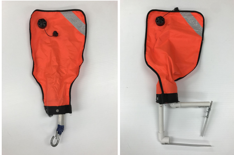
Figure 5: Modified lift bags used for retrieving the cannon (left) and the degraded tire (right)
