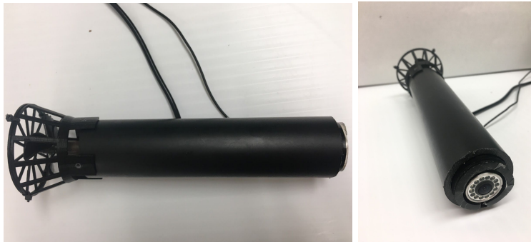
Figure 10: The Husky Explorer micro-ROV for drain pipe inspection
