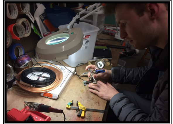
Figure 32: Modifying the fiber optic cable
