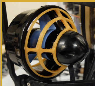
Fig. 4 - Shroud on the back of a Blue Robotics T200 thruster
