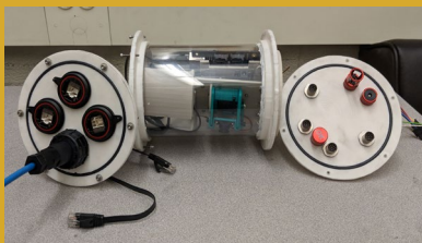
Fig. 10 - Initial version of logic enclosure showing connector and sensor placement
