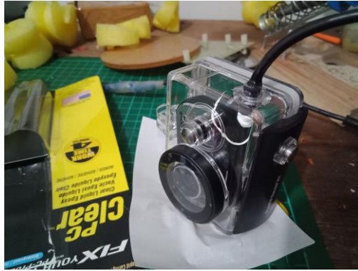
Fig 18. Sealed usb camera in yii waterproof case (Credit: Prabu)
