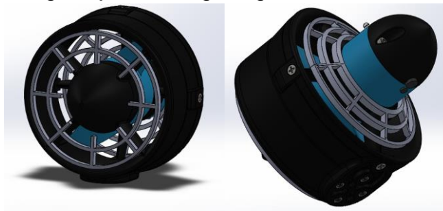
Fig 10. Thruster guard design for safety (Credit: Abyan)
