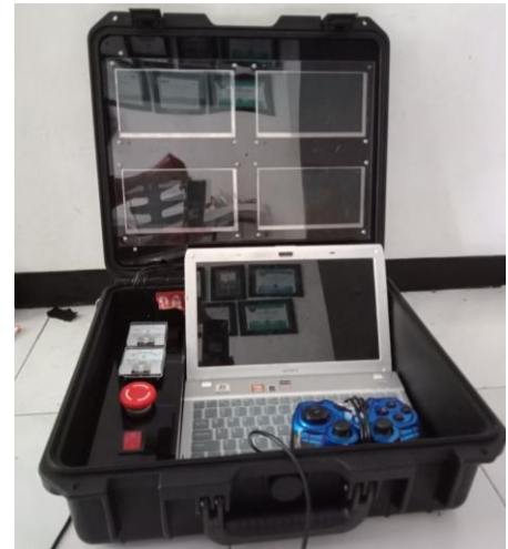
Fig 11. Ground Control System (Credit : Prabu)
