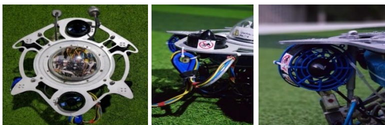
Figure (45): edges, Safe tether, bolts, and thrusters.
