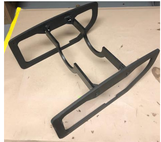
Figure 4: Completed laminate chassis frame
