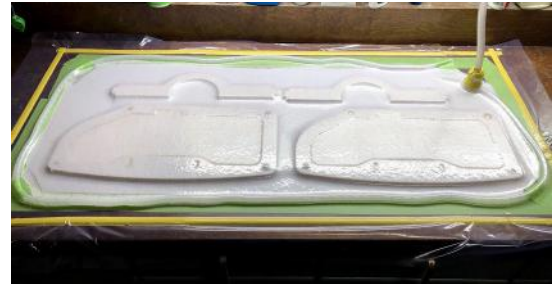
Figure 5: G-10 Laminate chassis frame being vacuum bagged
