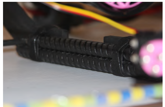
Figure 7: Rebar attached to the skids of the chassis
