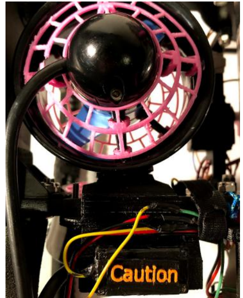
Figure 24: Caution signs installed on the motors
