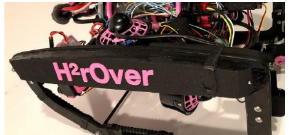
Figure 6: Buoyant high density foam attached to the H2rOver
