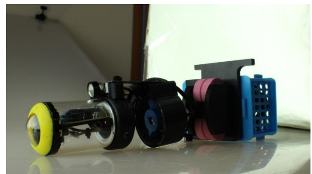
Figure 18. Automatic Tether Reeler with the Micro-ROV
