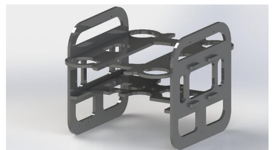
Figure 4. Render of the Matryoshka-ROV frame
