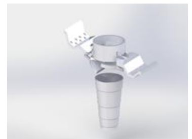
Figure 24a) First prototype of Mechanical Grout Inserter
