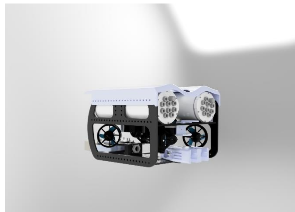
Figure 6 - ROV with microROV showing at the back
