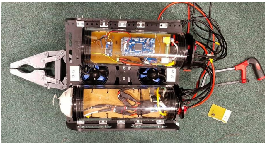
Figure 15 - top view of the ROV, showing some of the electrical systems such as the ESCs
