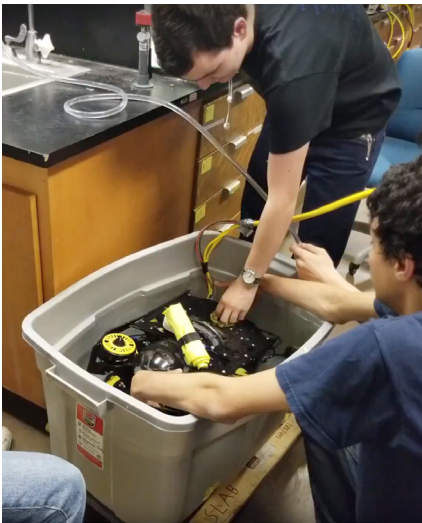
Fig. 23: Using a bin to test the ROV for leaks
