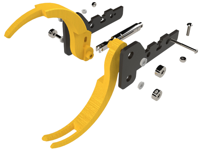
Fig. 8: An exploded view render of the large claw, with HDPE mount, piston, and gripper
