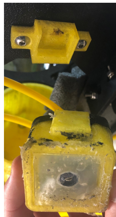
Fig. 19: Exteral camera detached, with magnetic mount visible above
