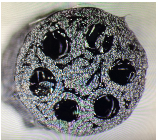
Fig. 18: 10x magnified view of a 16AWG TPU adapter
