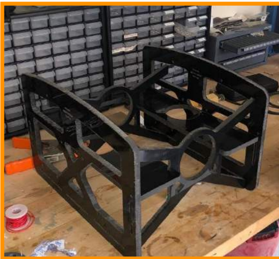
21-First test fit of hull panels
