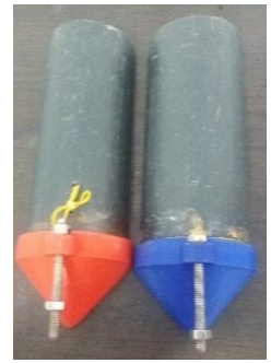
Figure 35: The grout tool
