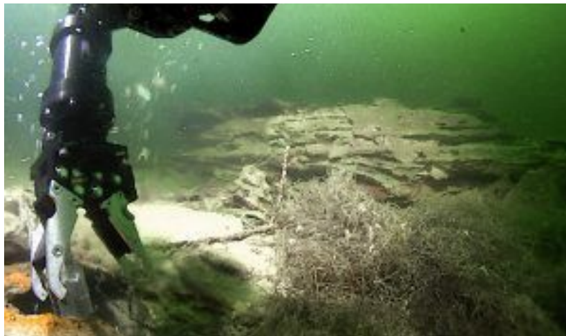
An ROV uses its claw to measure the temperature of a hydrothermal vent in Yellowstone Lake. Credit: Loalvo
