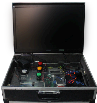
Figure 23: Topside Control Unit
