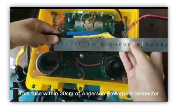
• The inside of the control box is does not have exposed wiring (ELEC-017R), the control box is neatly laid out with attention to workmanship (ELEC-022R), a separation and identification of 120VAC wiring from DC and control voltages (ELEC-023R). If AC wiring is not used in the control box, include a statement saying no AC is used. ----Satisfied
