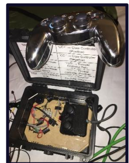
Figure 16: Inside view of the earlier stages of making the control box.
