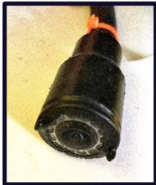
Figure 20: Waterproofed camera used on the ROV.
