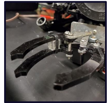
Figure 13: The 3-pronged claws utilized on the ROV. Photo by Nicholas Tassistro.
