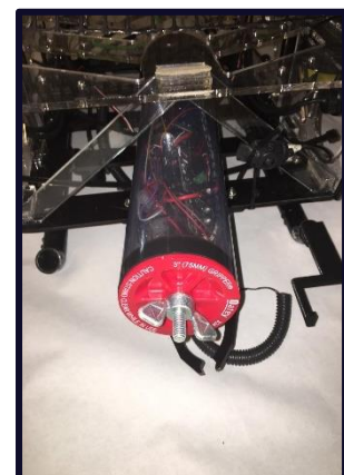
Figure 18: Tube containing the on-board electronics.
