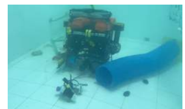
Figure 36: Micro-ROV retrieving a sediment sample by using Velcro hooks and Velcro loop successfully. (Image by Candy LEE)
