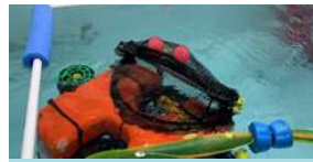
Figure 34: Plastic debris collector changes to a fish net and succeed in collecting ping-pong balls (Image by Candy LEE)
