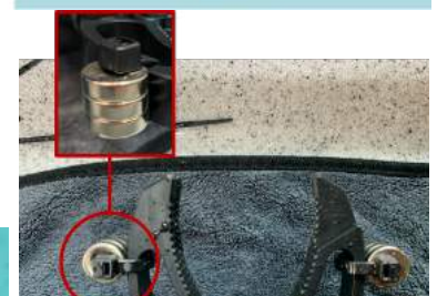
Figure 27: The pin falls from the main manipulator easily after removing from ghost net (Image by Candy LEE)
